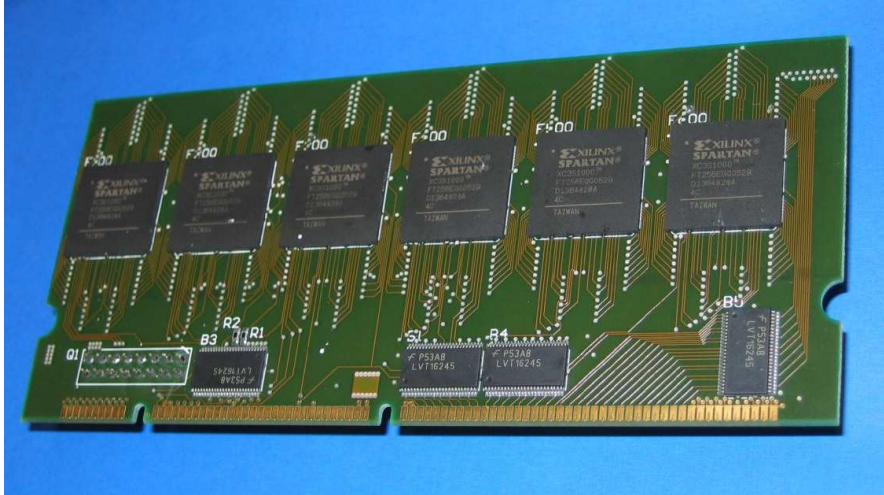
Figure 3: FPGA module (4-layer printed circuit board)
